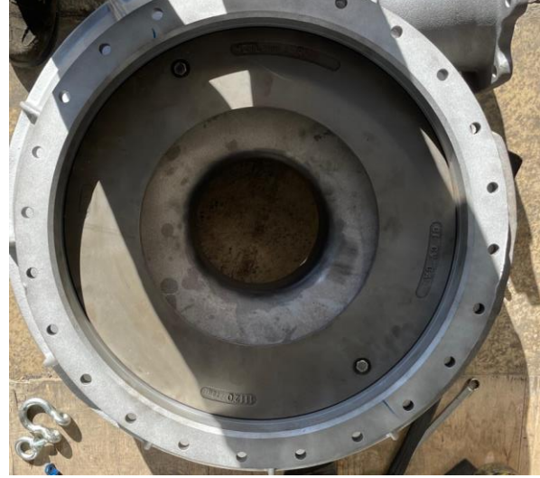
Fig. 4: Diffuser & Wall Insert (CT25 CV20 CA30)
